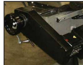
Y-Axis Drive Assembly. Driven by a powerful 27"lb (3.3 Nm) AC brushless servo motor (optional 41"lb., 4.6 Nm), this assembly features a tough and extremely durable one-piece machined casting.
